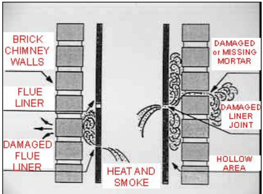
Cracks found in the structure caused by seismic activity are many times, small and tight fitting. These cracks are not always unobstructed nor allow the free passage of smoke as an open breach might do.
